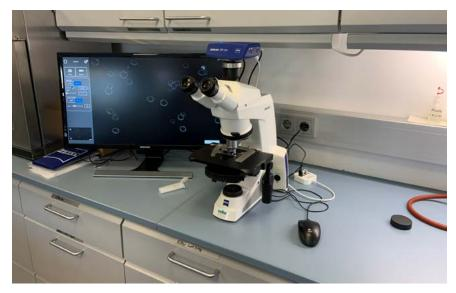
Figure 9 The ZEISS Axiolab 5 laboratory microscope provides high-contrast images of beer yeasts.
