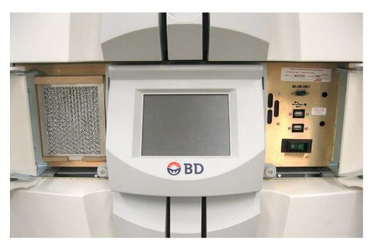
Figure 6-4 – Bottom Cabinet Air Filter (LCD bezel in place, access doors open)
