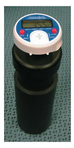
Figure 3-7 – Digital Thermometer
