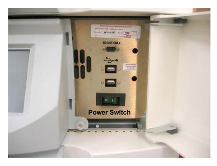
Figure 3-2 – Upper Instrument Power Switch
