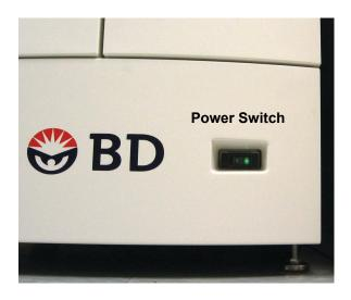
Figure 3-3 – Lower Instrument Power Switch
