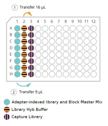
Figure 3. Overview of final plate setup
